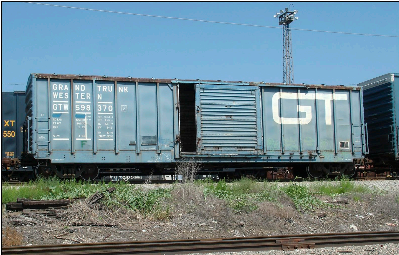
GTW 598370 was built 5/79 with improved Dreadnaught ends.
