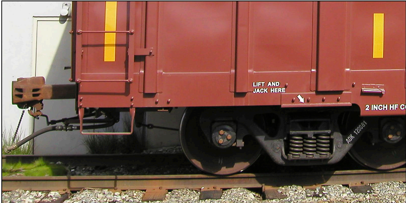
AOK 120081 (6663 cubic feet) was built 12/03 with straight side sills and the signature Gunderson Concarril 3-piece jack pad.
