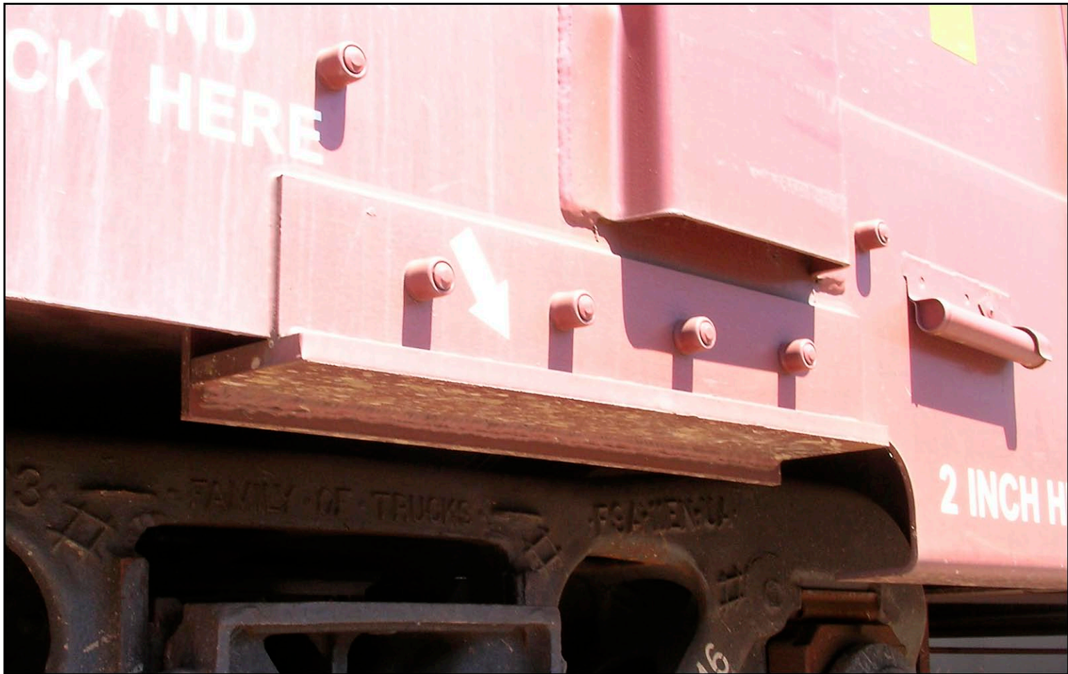
Another angle of a Gunderson Concarril jack pad, this one on AOK 120016.
